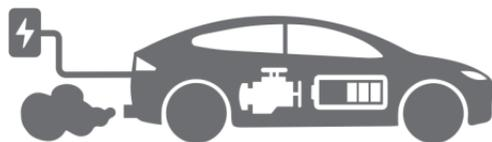
**Plug-in Hybrid Electric Vehicles (PHEVs):** PHEVs are fossil fuel-powered vehicles driven by an internal combustion engine that also have an electric motor. PHEVs operate on electricity until the battery is nearly depleted, then the gasoline-powered engine activates to provide power. Like Battery Electric Vehicles, PHEVs must be plugged in to an EV charger to charge the battery.
